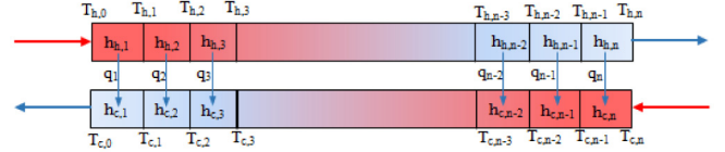
Fig. 5. Recuperator representation by discretizing into several segments.
