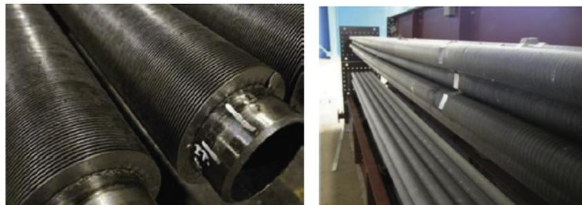
Fig. 3. Finned tube heat exchanger tube bundles.
